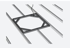
**3** Let the cable coming from the remote 24 VDC driver pass trough the hole. Screw your existing plasterboard to the structure perimetrally.
