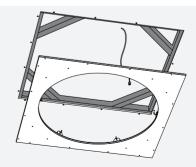
**5** Screw the plasterboard supplied on your new metal structure.
