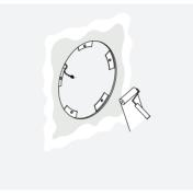
**9** Connect the power cable, put the panel at the right position and turn it clockwise checking that the panel is well fixed before of leaving it.
