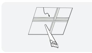
**1** Cut the square and remove the metal parts behind if present.
