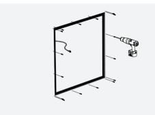
**2** Let the current cable coming from the 24 VDC remote driver pass trough holeand position the pre-drilled metal clips supplied.
