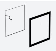
4 Position the plasterboard fastening panel (supplied).
