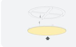
**7** Dress the magnetic finish belt plate around the thickness of panel. If the belt seems too short, adjust the light circle position moving it a little bit; there is tolerance for this operation.
