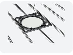
**6** Put the adhesive mesh (not supplied) around the seam and plaster.
