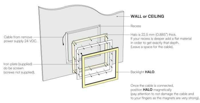
Note: The cup of screws must be less deep then 3mm.
